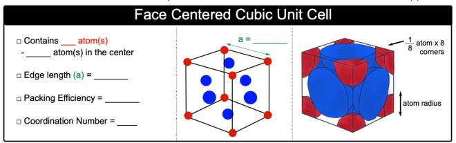
**EXAMPLE:** Silver adopts a face-centered cubic unit cell structure. Illustrate how the number of atoms per unit cell for the silver atom are obtained.
